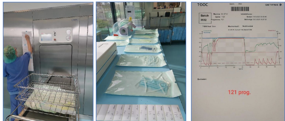
Fig 1. Autoclave procedure with Halyard laminate bags. Left, laminated bags entering the autoclave. Middle, masks are wrapped in laminate. Right, the 121 °C steam sterilization program as used for face mask sterilization.
