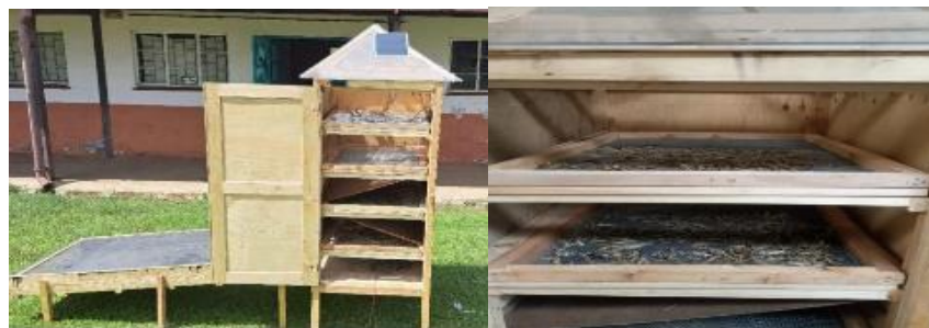
Fig. 4. Dryer assembly and tray decks
